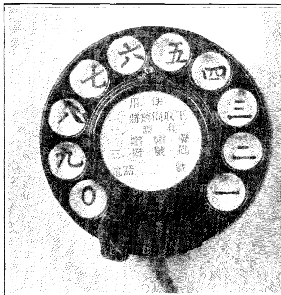
Figure 4—Calling Dials of Special Design. They are marked either with Arabic numerals or Chinese characters.
