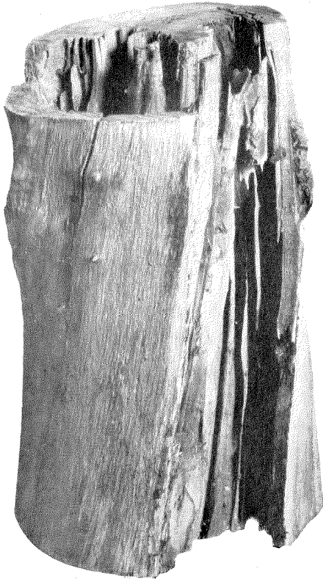
Figure 4—Piece of an Untreated Pole Butt Ravaged by Insects.
