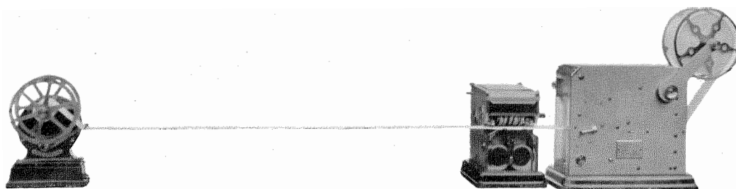
Figure 13—Register, Time Stamp and Take-up Reel as Mounted at Fire Station.
